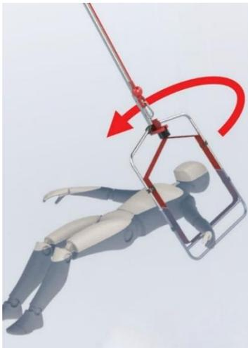
**Image A9:** Start under one arm, up to the arm pit and rotate the hoop over the head
