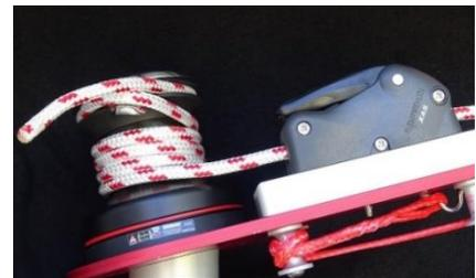
**Image D22 – Line brake closed, line wrapped, in winch jaws. Tailed off the chrome tailing arm, ready to lift**
