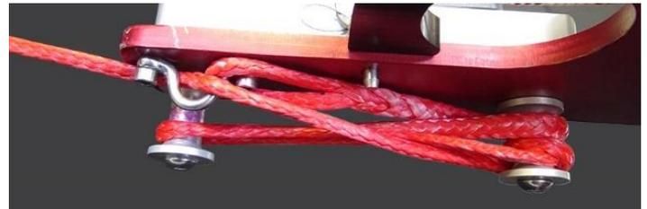
**Image E21 – Eye strap re-attached with the tension line secured inside the eye**
