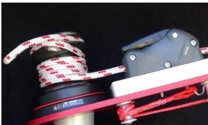
**Image D37 – Line brake closed, line wrapped, and in winch jaws. Tailed off the chrome tailing arm, ready to lift**
