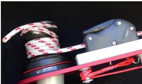
**Image E24 – Line brake closed, line wrapped, and in winch jaws. Tailed off the chrome tailing arm, ready to lift**
