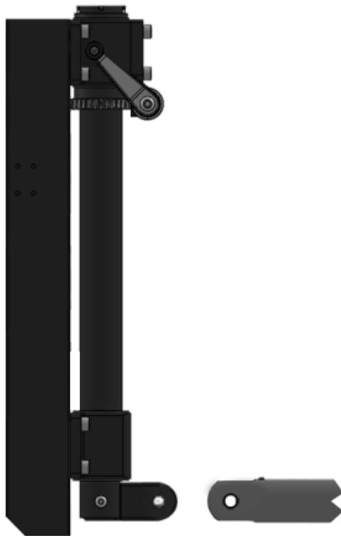
**Image E7 – Side view of base with davit boom ready to insert**
