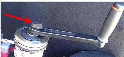
**Image D23 – Winch Handle with thumb lock**
