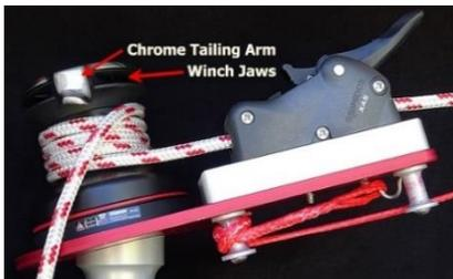
**Image D21 – Line brake open, line out of jaws, ready to ease the line off the winch and lower the dummy to the deck**
