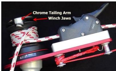
**Image E12 – Line brake open, line out of jaws, ready to ease the line off the winch and lower the PIW to the deck**
