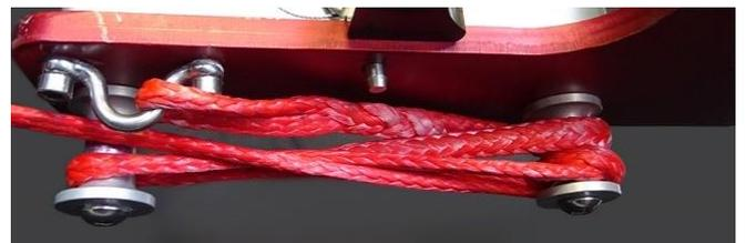
**Image D29 – Wraps on buttons with a half hitch finish**
