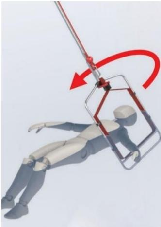
**Image C10:** Start under one arm, up to the arm pit and rotate the hoop over the head
