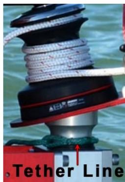
**Image D15 - Tether Line (Not included) on winch collar**
