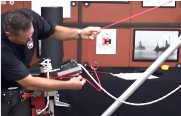
**Image E17 – Holding Tension Line to lift Davit boom to approximately 45°, while wrapping the Tension Line round the adjusting buttons under the winch plate**
