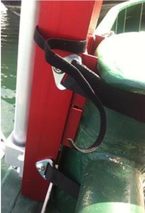
**D4 - This shows how it should fit, not bottoming out and touching the bitt between the red feet**
