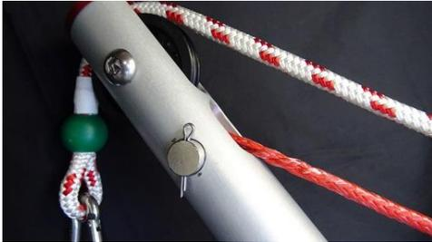
**Image D19 – Tension line around pin inside the boom with cotter pin inserted**
