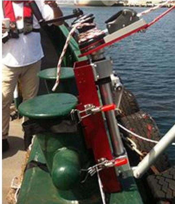
**D5 - This shows a properly installed Rescue Davit, side stabilizers are more easily seen on back view of davit on Images D11 & D12**
