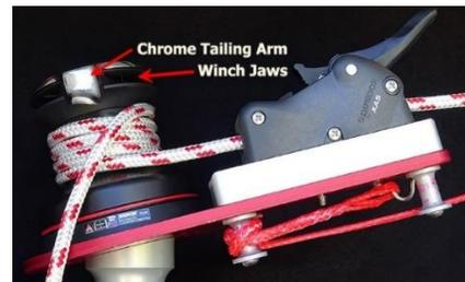
**Image D38 – Line brake open, line out of jaws, ready to ease the line off the winch and lower the dummy to the deck**
