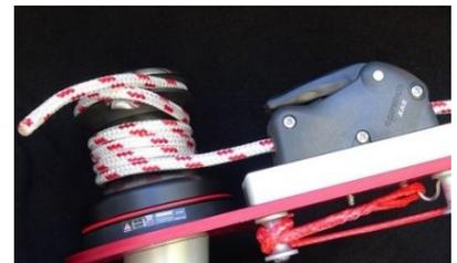
**Image E13 – Line brake closed, line wrapped, in winch jaws. Tailed off the chrome tailing arm, ready to lift**
