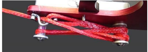
**Image D31 – Eye strap re-attached with the tension line secured inside the eye.**
