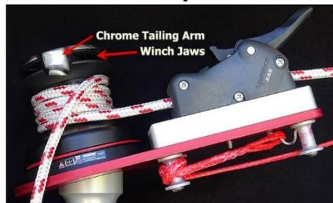
**Image E25 – Line brake open, line out of jaws, ready to ease the line off the winch and lower the dummy to the deck**
