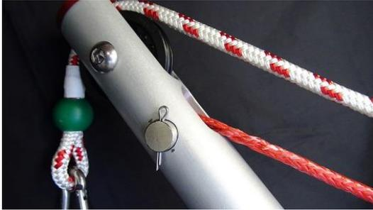
**Image E10 – Tension line around pin inside the boom with cotter pin inserted**
